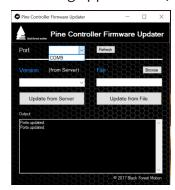
Once the correct port is selected, you can select the latest firmware version from the server. Click on "Update from Server" to install the firmware.
