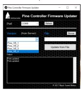
As soon as the output confirms the process successfully, the firmware was installed. To use the controller with the new firmware, it must be restarted. To do this, simply disconnect the power supply.
